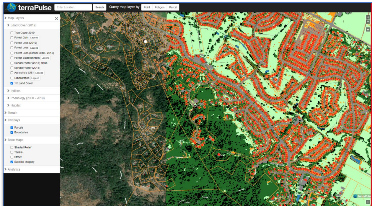
The terraView dashboard showing the 1-meter resolution terraPulse Land Cover Type layer over a wildland-urban interface in Sonoma County, California. Cover types are: building (red), pavement (gray), tree (dark green), grass/herb (light green), water (blue).
